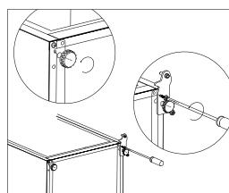
8. Unscrew and remove the bottom hinge pin, turn the bracket over and replace it.
