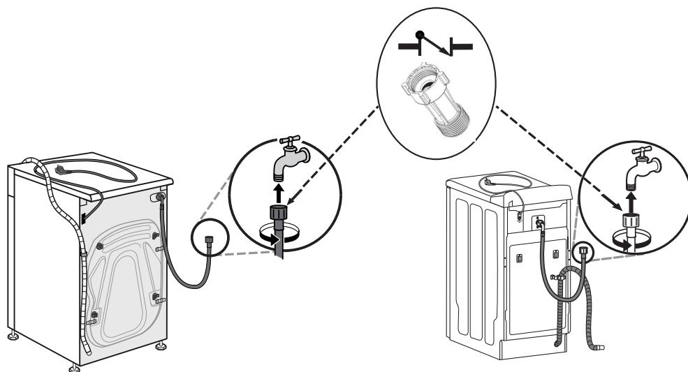
**EN** According to the relevant EN 61770 / DIN standards, the appliance must be connected to a water supply system with a check valve, service spare part number C0084677 or equivalent.
