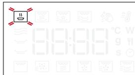
Turn the *knob* to select from amongst the subfunctions available on the right-hand display and then press to confirm. The sub-function in selection will blink until its confirmation.
