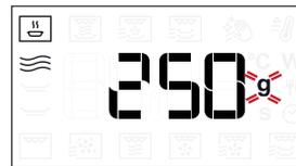
When the default setting appears on the display and the icon flashes, turn the *knob* to set the weight and then press to confirm.
