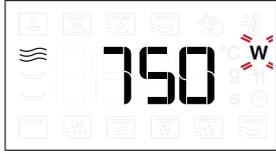
When the **W** icon flashes on the display, turn the *knob* to adjust the power setting and then press **Ⓔ** to confirm and continue to alter the settings that follow (if possible).
