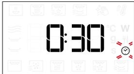
When the **⌚** icon flashes on the display, use the *knob* to set the cooking time you require and then press **Ⓔ** to confirm.
