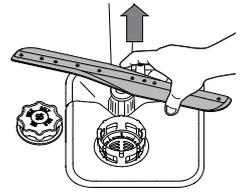
The lower spray arm may be removed by pulling it upwards.
