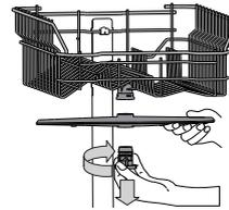
To remove the upper spray arm, turn the plastic locking ring in a clockwise direction.
