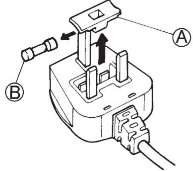
1. Remove the fuse cover (A) and fuse (B).
