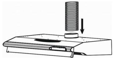
Use an outlet exhaust duct with: - minimum indispensable length; -Minimum possible bends (maximum angle of bend: 90°); -certified material (according to local, building & fire regulations); and as smooth as possible inside. It is also advisable to avoid any drastic changes in duct cross-section (recommended diameter: 125mm).
