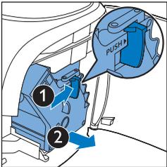
4 Press the PUSH button (1) and pull at the grip of the brewing unit (2) to remove it from the machine.
